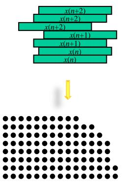
• A carry-propagate adder finally reduces the *y* filter output to a single word
