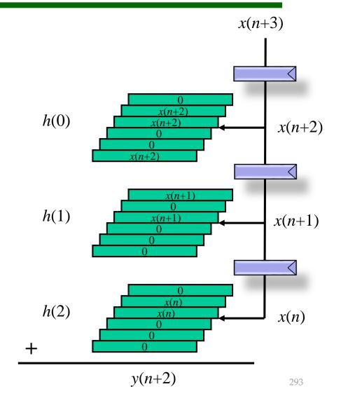
• In the common case when the *h* coefficients are fixed, there is of course no change and no downside if the "always zero" partial products are removed
