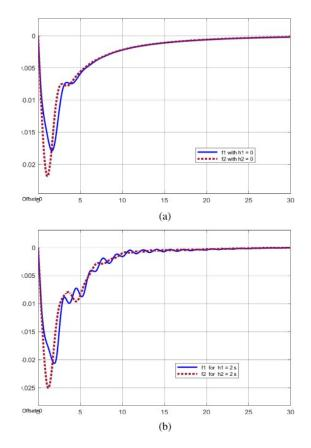
Fig. 5. Frequency deviation outputs  $f_1$  and  $f_2$  with load disturbances  $v_1 = v_2 = 0.01$ , with no time delays and with time delays of  $h_1 = h_2 = 2$  s using PID controllers.
