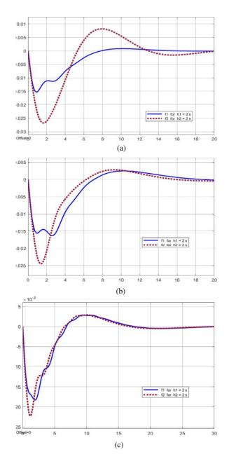
Fig. 4. Frequency deviation outputs  $f_1$  and  $f_2$  with load disturbances  $v_1 = v_2 = 0.01$ , with time delays of  $h_1 = h_2 = 2$  s.
