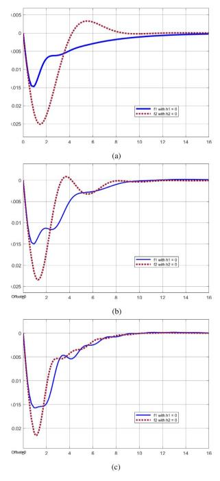
Fig. 3. Frequency deviation outputs  $f_1$  and  $f_2$  with load disturbances  $v_1 = v_2 = 0.01$ , with no time delays  $h_1 = h_2 = 0$ .
