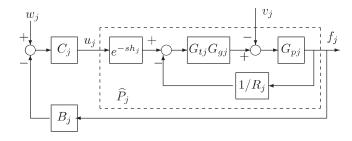
Fig. 1. Closed-loop single-area power system  $\mathcal{S}_j$ .
