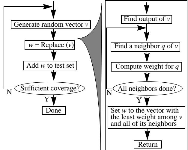
Figure 5 Flowchart of BT for multiple-output circuits.
