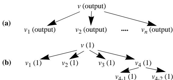
**Figure 4** Tree diagram for single-output circuits: (a) general case and (b) an example.
