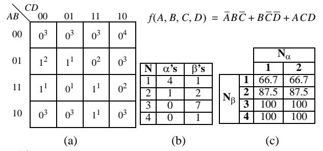
**Figure 2** A four-input circuit: (a) K-map, (b) vector distribution, and (c) fault coverage.
