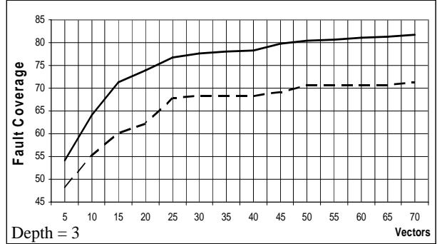
Figure 6 Fault coverage as a function of the number of vectors for the circuit c1908.
