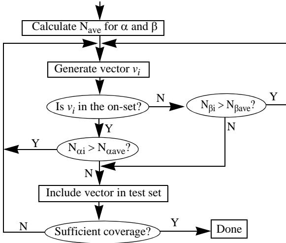
**Figure 3** Flowchart of BT for single-output circuits using an average.
