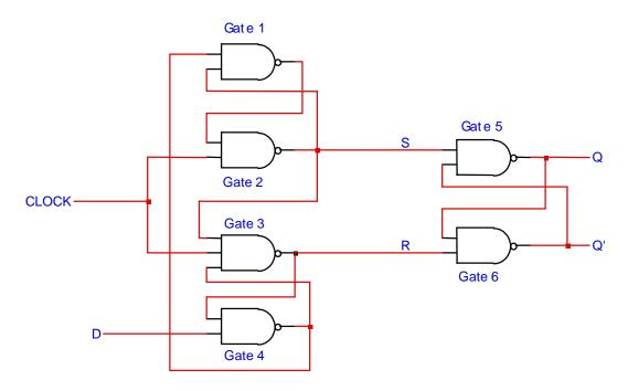
Figure 5: D-type positive-edge-triggered flip-flop
