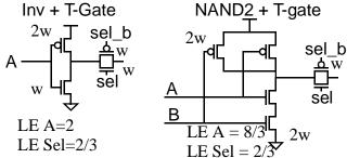
doubles the resistance of the gate without changing the input capacitance.
