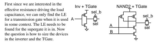
To start we need to know whether we should consider sel and sel\_b two different signals, or should we add the cap together. The answer is described in more detail in the next section, and turns out that the logical effort of a splitter (creates A and A\_b) is only slightly greater than one. So the logic effort should be considered by only looking at the 'sel' input.
