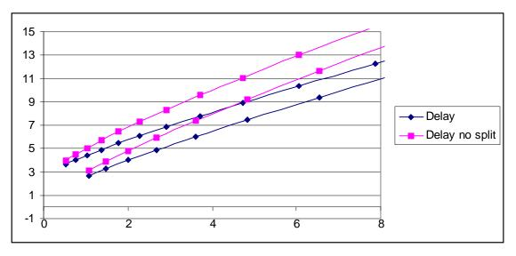
The blue curves (with diamonds) are the result of splitting the first inverter. If the inverter is not split (the first technique) you get the pink (squares) curves. The lower curves are the results you get if you ignore the parasitic delay, the upper curves are the results if the self loading is equal to its gate capacitance.
